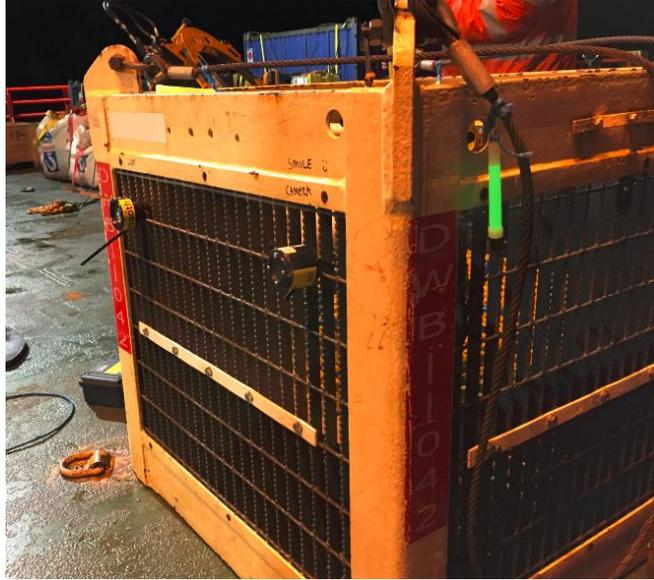
Seatooth Video MkII Wireless Subsea cameras mounted on to Skid
