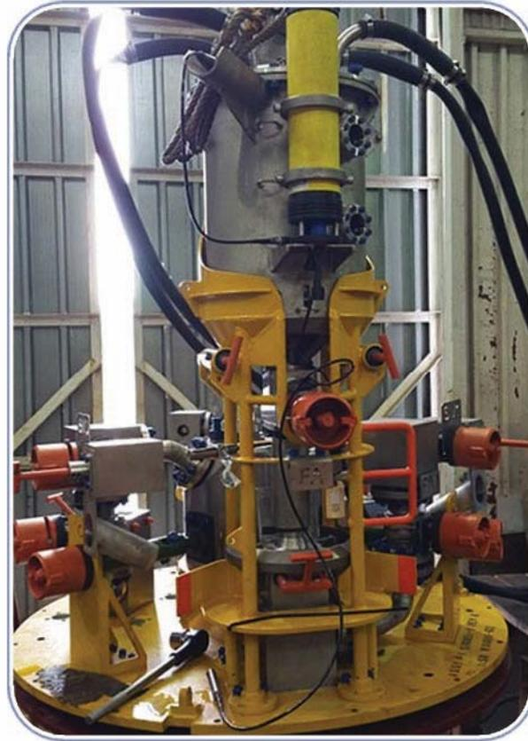
Submarine Mineral Genesis Monitoring System with WFS Seatooth® S100 and other telemetry equipment at flow test
